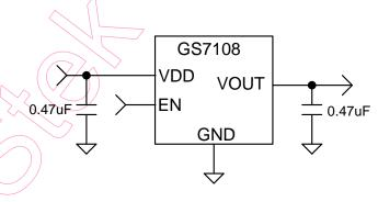
Figure.1 Typical Application of GS7108
